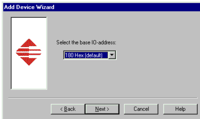
Figure 6. Set the I/O Base Address to 180.
